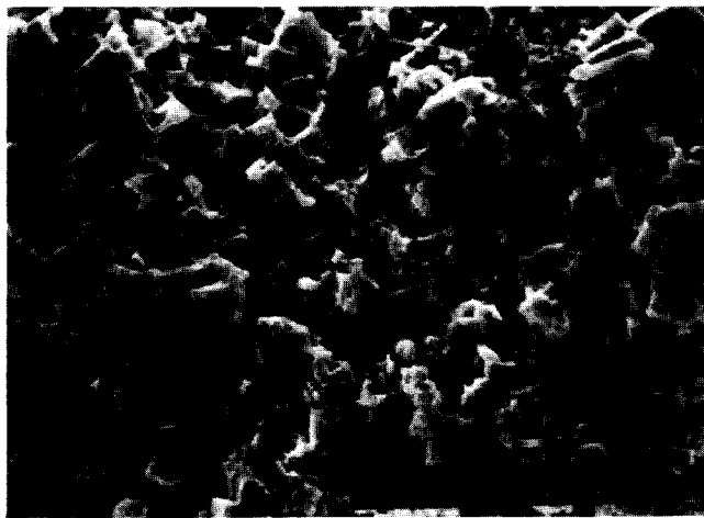
Fig. 5 Dissolution of grain boundaries and some intergranular attack on alloy 1 in the H-18 temper.
